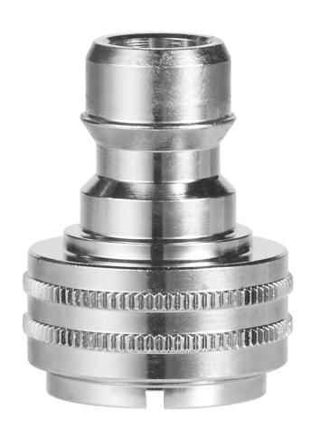
Fits water tap with  $\frac{1}{2}$ ",  $\frac{3}{4}$ " or M22 mm outside thread. When the bush is removed, the coupling fits a 3/4" external thread. When the bush with the 2 small notches is turned it fits a 1/2" external thread When the bush with the 2 small notches is turned down it fits a M22 mm external thread.
